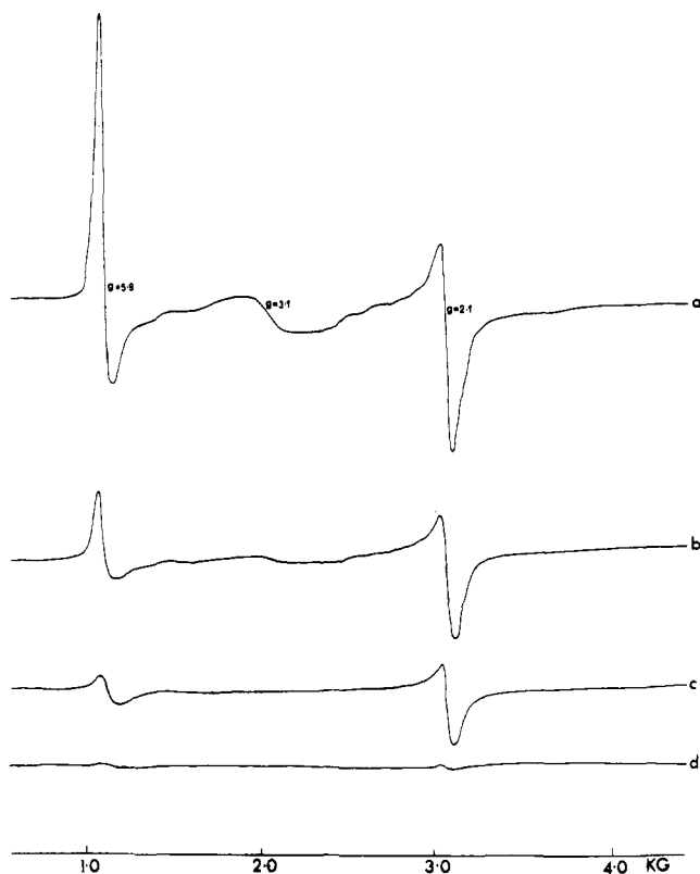
Figure 2. ESR spectra of 1 in frozen solution (5% MeOH in \text{CHCl}_3 ) at various temperatures: (a) 4.2 K; (b) 15 K; (c) 27 K; (d) 40 K.
